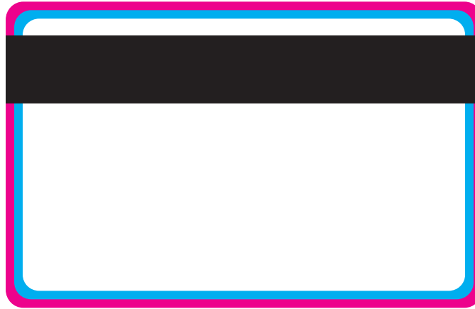
WITH 3-TRACK FLUSH MAG STRIPE \frac{1}{2} " (.5") HEIGHT \frac{3}{16} " (.1875") DISTANCE FROM EDGE
