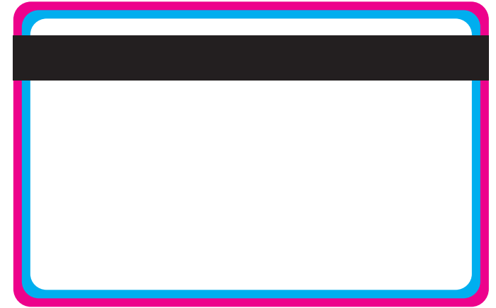
WITH 2-TRACK FLUSH MAG STRIPE \frac{33}{100} " (.33") HEIGHT \frac{3}{16} " (.1875") DISTANCE FROM EDGE
