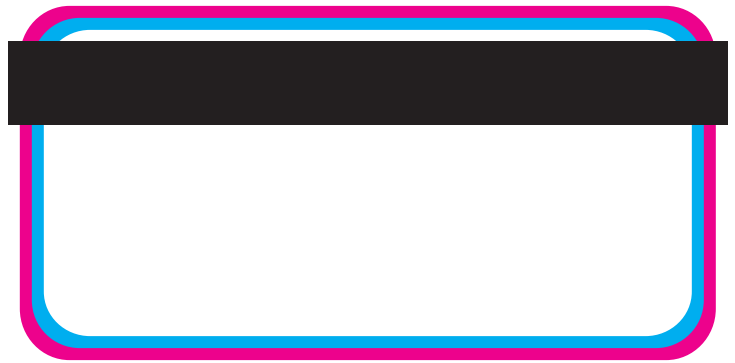
WITH 3-TRACK ROLL-ON MAG STRIPE \frac{7}{16} " (.4375") HEIGHT (.1227") DISTANCE FROM EDGE
